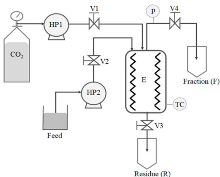
Figure 1. A schematic flow diagram of a continuous SC-CO<sub>2</sub> fractionation system. E: extractor; Feed: sample feed; HP1: super-critical CO<sub>2</sub> pump; HP2: high-pressure liquid pump; TC: temperature gauge; P: pressure gauges; V1-V4: high-pressure valves.
